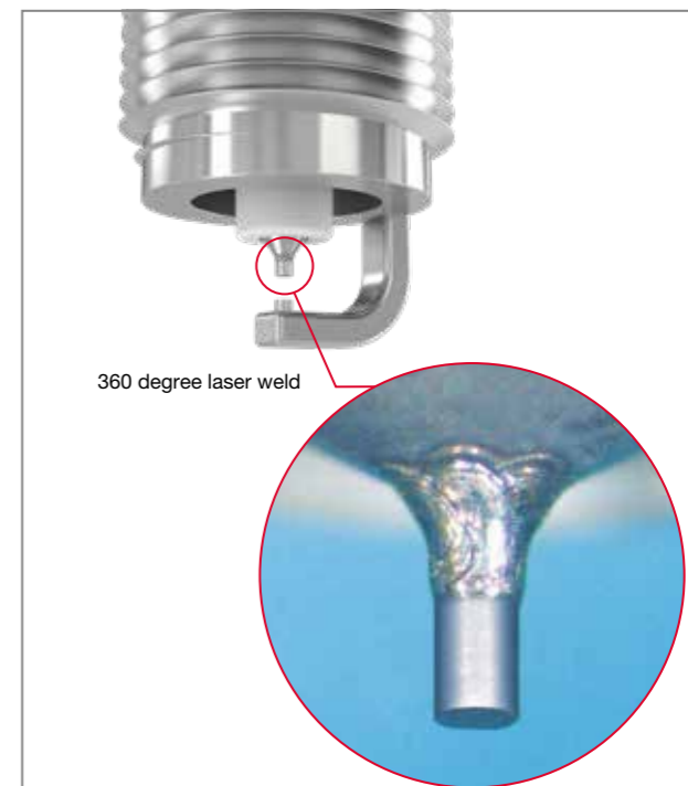
Fig 7.6 Iridium centre electrode – 0.4mm diameter
